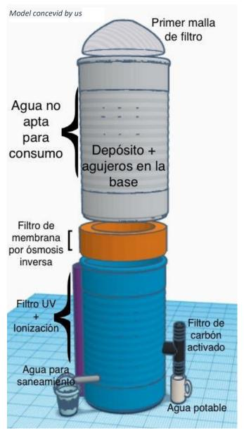
The model we have devised consists of several components that work together to eliminate a wide range of water contaminants. Prefilters are the first components in the reverse osmosis process and are used to remove large particles and organic matter before the water enters the purification process.
