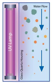
charged molecules that can be removed through ion exchange. The UV lamp is used in conjunction with an ion exchange process to maintain water quality. This method can produce water with very low levels of organic carbon and bacteria.
