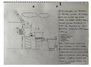
PVC pipes for storing the filtered water. The necessary nutrients for plant growth are provided through the application of liquid worm humus, a natural fertilizer. To ensure proper oxygenation of the water, an air recirculation pump is used, which allows for the circulation of water so that plants can absorb the necessary nutrients and oxygen for their optimal development.
