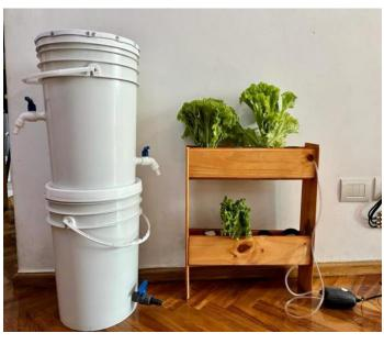
filtration. This prototype not only filters the water but also allows for its storage for later use. In this process, after all sediment has been filtered, the water is stored in a container, which is considered as "sanitation water", as it can be used for cleaning, irrigation (in our case, for supplying the hydroponic crops), or even toilet flushing. It then goes through a natural filtration process before being stored in a second tank. The obtained water is potable and suitable
