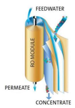
A reverse osmosis system is a highly effective method for water purification. The process involves the circulation of water through a membrane under pressure in a cross-flow manner, removing up to 99% of impurities.
